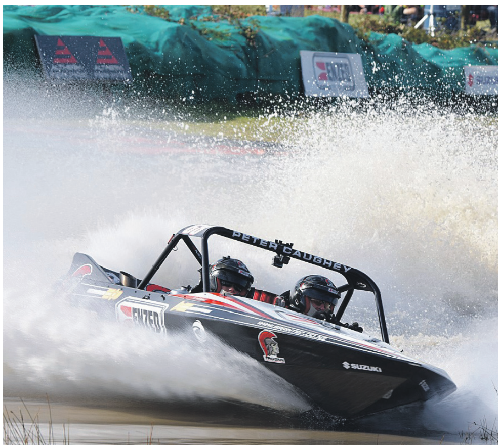
SuperBoats like Peter Caughey's ENZED Sprintec racer use fuel injection and open trumpets, which don't gel well with heavy rain – and the SuperBoat class was called off after three qualifying runs. Photo by Ian Thornton.
