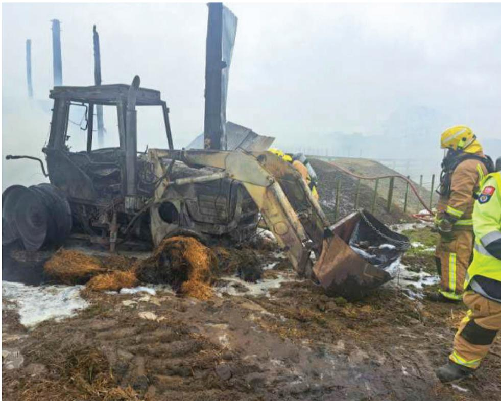
Please take a bit of time to check under the hood for any hay around the engine area each morning.
