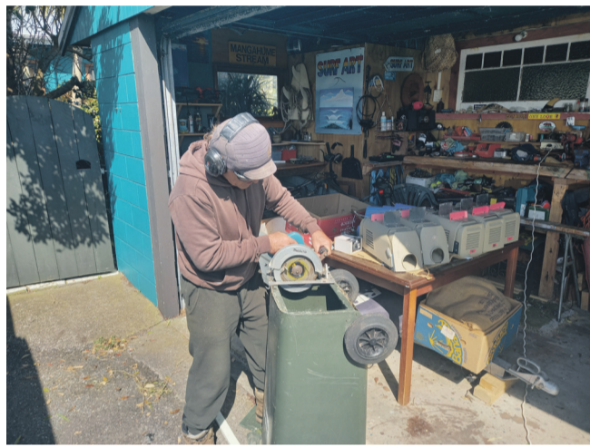
Cutting the bottom off the bin.
